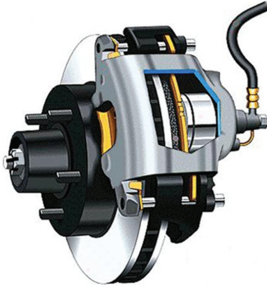
A disc brake (image courtesy Paul Turnbull, SEMTA, Watford, UK. www.gcseinengineering )
